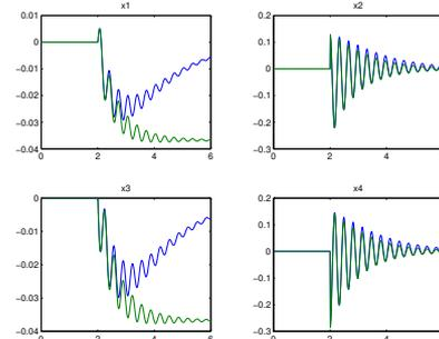
When only velocity is penalized, a static position error remains
