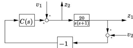
With  $P(s) = \frac{20}{s(s+1)}$ , the transfer matrix from  $(v_1, v_2)$  to  $(z_1, z_2)$  is
