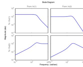
Nonzero static gain in  $\frac{P}{1+PC}$  indicates poor disturbance rejection
