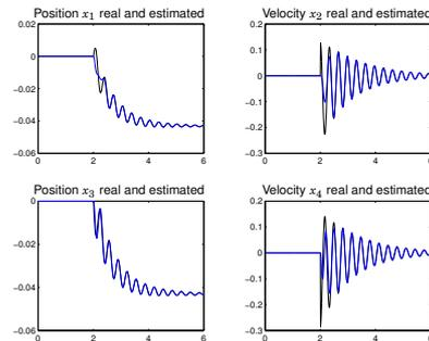
The measurement  $y_1$  is not trusted, so the estimate of  $x_1$  slows down.
