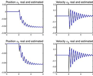
A Kalman filter estimates the states using measured positions.
