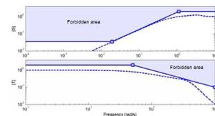
We will see that if there are zeros in the right half plane (so called *nonminimum phase zeros*) and/or unstable poles in the loop gain  $L = PC$ , this will put constraints on what specifications  $W_S$  and  $W_T$  we can satisfy.
