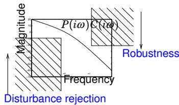
We will have the cross-over frequency  $\omega_c$  with stability margins  $A_m$  and  $\phi_m$  in the range between "low" and "high fq".
