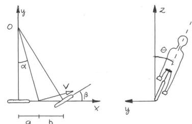
$$J \frac{d^2\theta}{dt^2} = mg\ell\theta + \frac{mV_0\ell}{b} \left( V_0\beta + a \frac{d\beta}{dt} \right)$$
