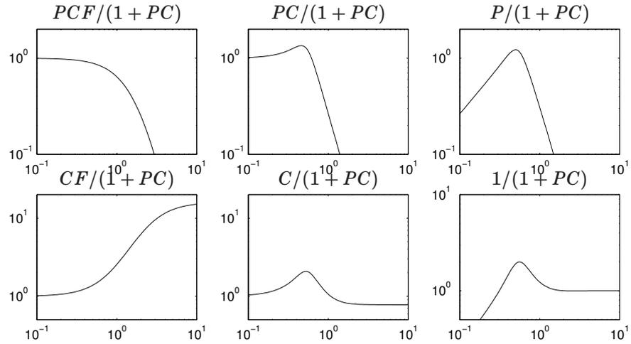
**Figure 4.3** Frequency response amplitudes for  $P(s) = (s+1)^{-4}$ ,  $C(s) = 0.775(s^{-1}/2.05 + 1)$  when  $F(s)$  is designed to give  $PCF/(1+PC) = (0.5s+1)^{-4}$
