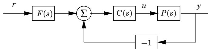
Figure 4.8 The feedforward filter  $F(s)$  is used to improve the response to reference signals
