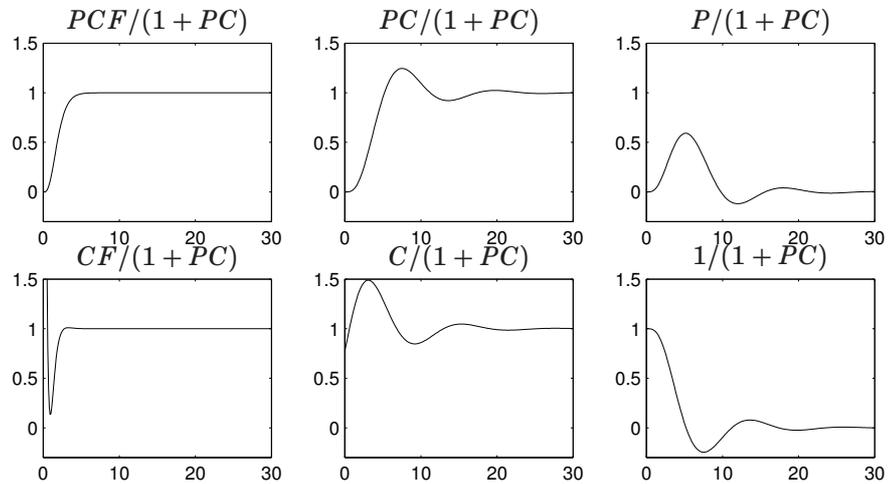
**Figure 4.4** Step responses for  $P(s) = (s+1)^{-4}$ ,  $C(s) = 0.775(s^{-1}/2.05 + 1)$  when  $F(s)$  is designed to give  $PCF/(1+PC) = (0.5s+1)^{-4}$
