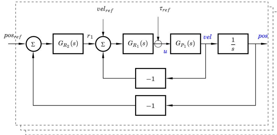
**Figure 4.9** Cascaded controller for servo control with feedforward control of velocity references and torque references, consistent with the desired position references (generated together).
