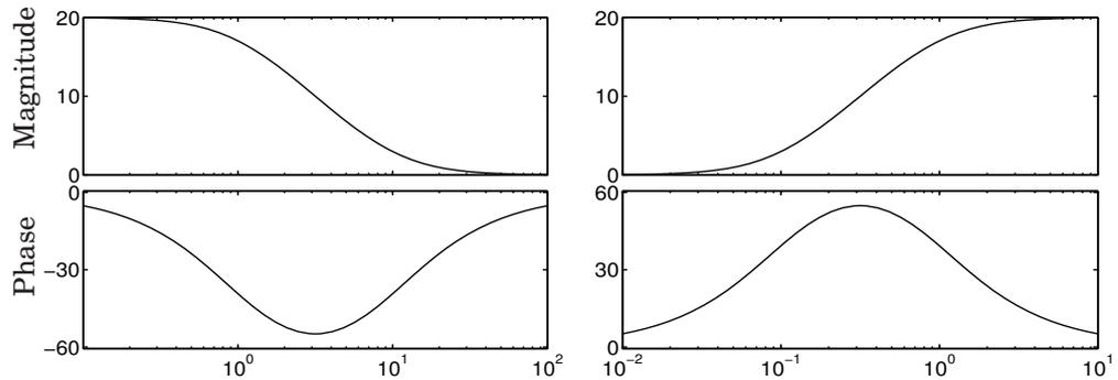
**Figure 4.6** Bode diagrams for lag compensator  $\frac{s+10}{s+1}$  (left) and lead compensator  $\frac{10s+1}{s+1}$  (right)
