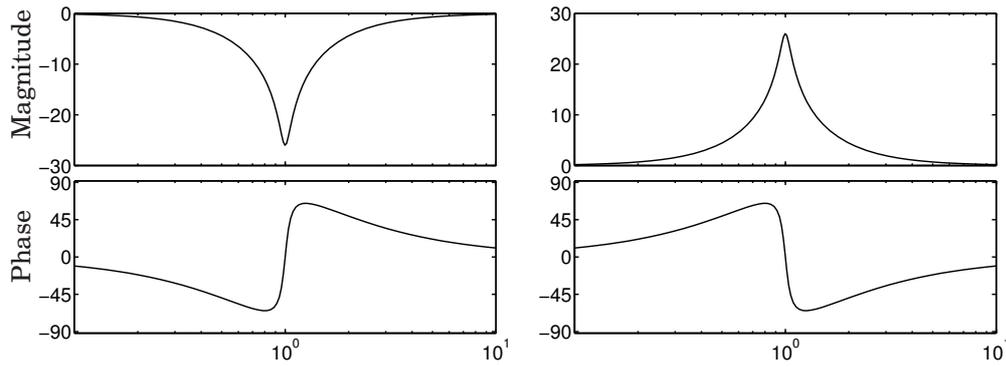
Figure 4.7 Notch compensator  $\frac{s^2+0.1s+1}{(s+1)^2}$  (left) and resonant compensator  $\frac{(s+1)^2}{s^2+0.1s+1}$  (right)
