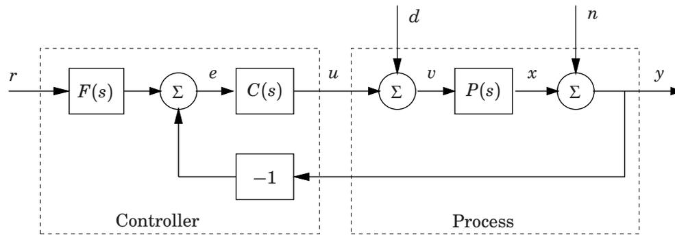
Figure 4.2 A Controller with two degrees of freedom
