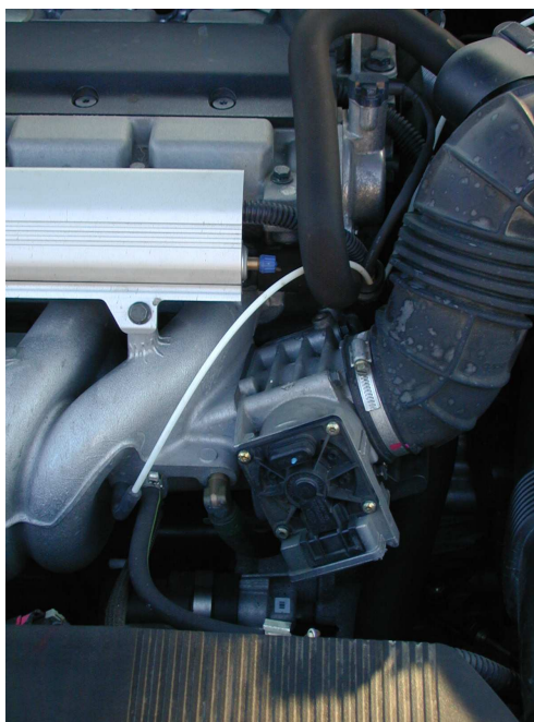
Figure 1 The throttle unit used in modern Volvo engines. By controlling the angular position of the circular plate inside the pipe, different amounts of air are fed into the engine. The position of the throttle in the overall Volvo engine system is shown in Figure 15 at the end of this manual.
