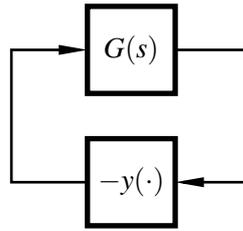
**Figure 4** The setup for the simulation in problem 3.b, where  $y(\cdot)$  is the relay described in (2).
