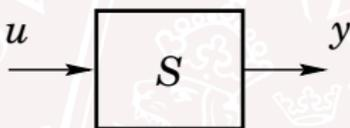
The gain  $\gamma$  of  $S$  should tell what is the largest amplification from  $u$  to  $y$
