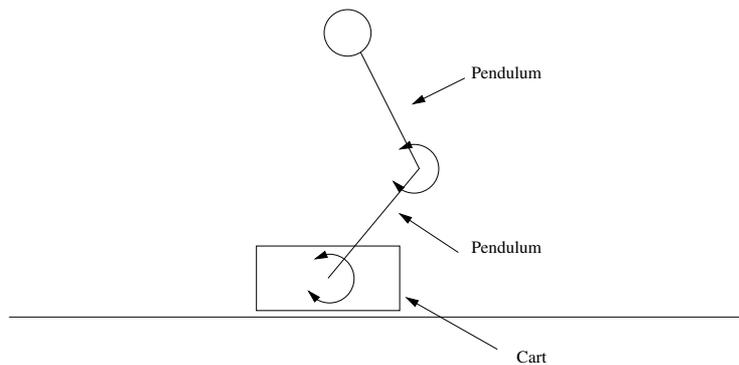
**Figure 1** The double pendulum. Two pendula in series are attached to a moving cart.
