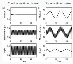
Sampling of high-frequency measurement noise may create new
