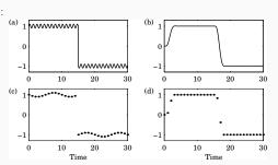
(a), (c):  $f_1=0.9$  Hz,  $f_N=0.5$  Hz  $\Rightarrow f_{alias}=0.1$  Hz
