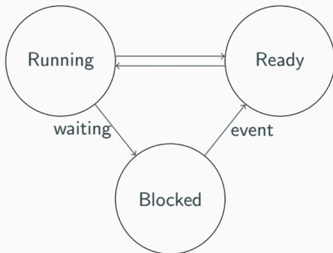
When `WaitTime/WaitUntil` is called: process moved from Running to Blocked (moved from ReadyQueue to TimeQueue). When time has passed: process moved from Blocked to Ready (done in the `Clock` procedure).
