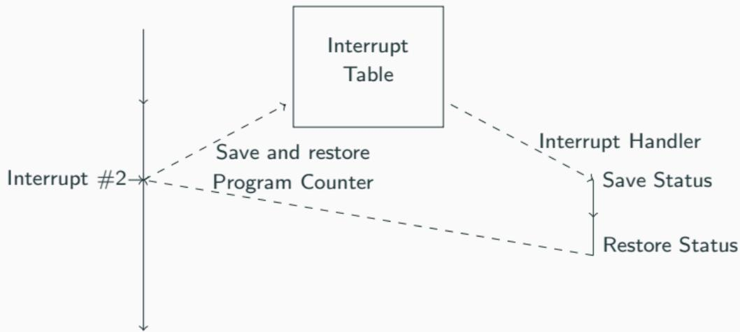
The Interrupt Table contains a mapping between the Interrupt Number and the Interrupt Handler that should be called. The interrupt number is known as the Interrupt Request (IRQ).
