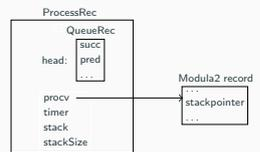
In the global data area, there are two pointers: ReadyQueue (pointer to a double linked list of processes that are ready to run) and running (pointer to the currently running process). For each process:
