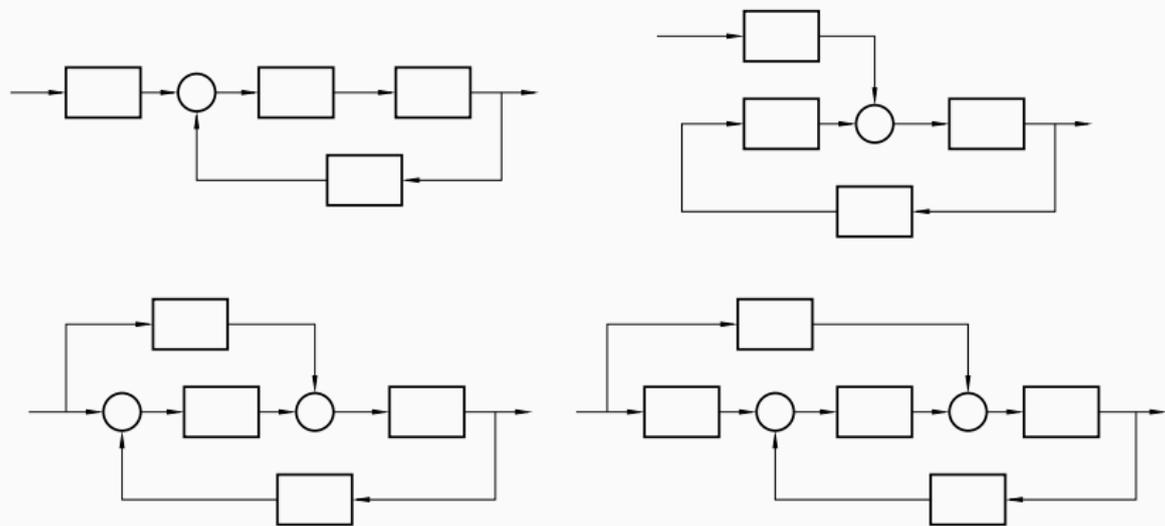
For linear systems, all these structures are equivalent
