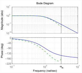
The hold circuit can be approximated by a delay of h/2
