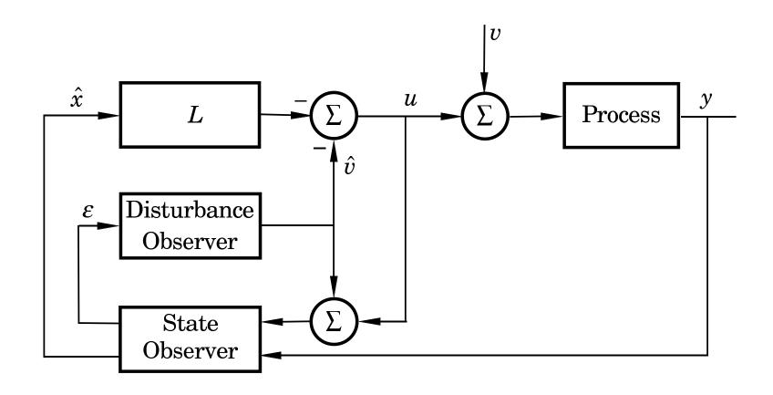
The disturbance estimator is integrating the prediction error of the observer.
