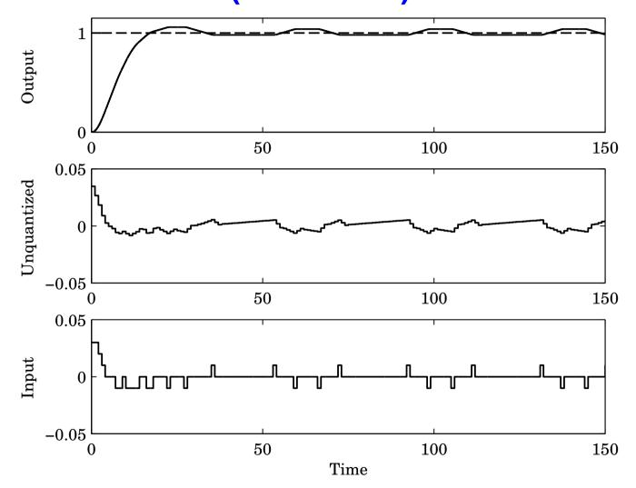
Limit cycle in process input with period 39 s, ampl. 0.01
