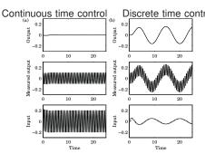
Sampling with high frequency measurement noise may create new frequencies!
