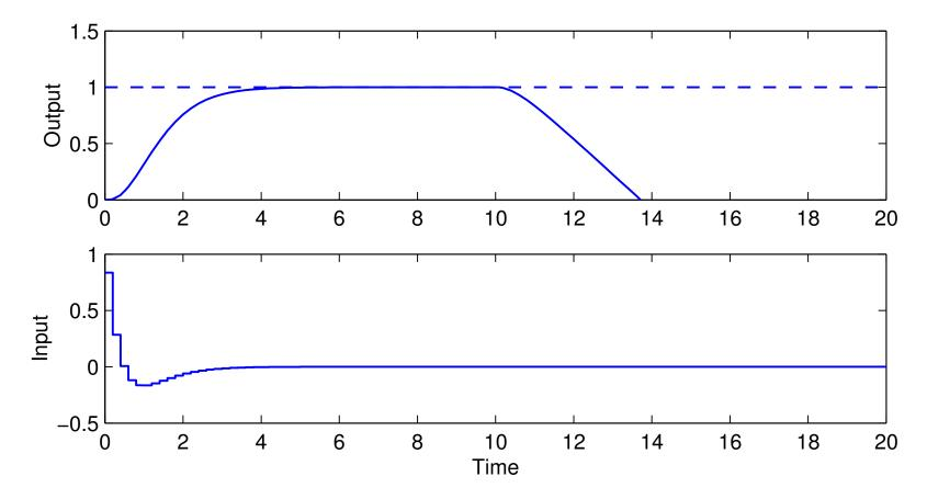
Does not work at all – the feedback is needed to handle the load disturbance
