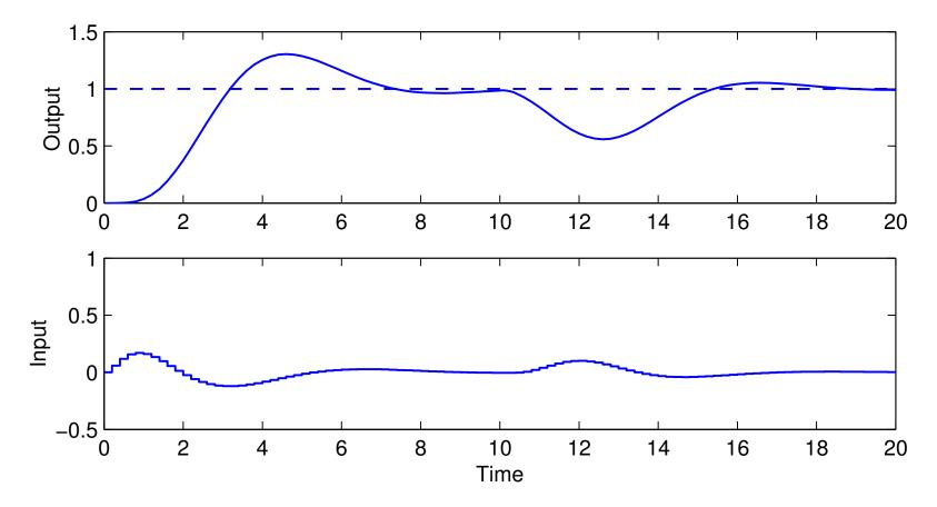
Does not work very well – the feedforward term is needed to get the desired reference step response
