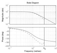
For slow signals, the hold circuit is approximately a  $\hbar/2$  delay. For fast signals, the hold circuit destroys the sinusoidal shape.
