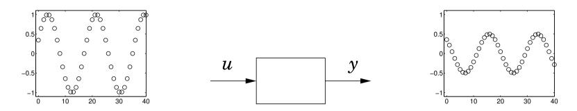
Given a stable system H(z), the input  $u(k) = \sin(\omega k)$  will, after a transient, give the output
