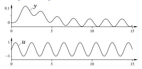
Given a stable system G(s), the input  $u(t) = \sin \omega t$  will, after a transient, give the output
