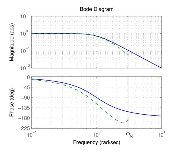
For slow signals, the hold circuit is approximately a h/2 delay. For fast signals, the hold circuit destroys the sinusoidal shape.
