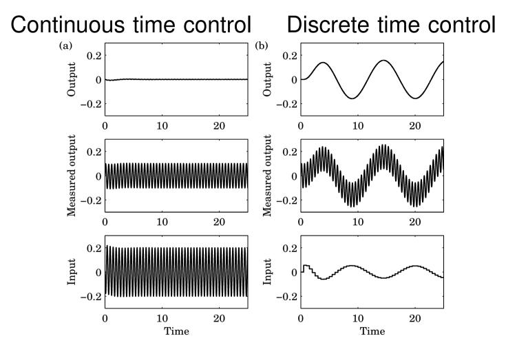
Sampling with high frequency measurement noise may create new frequencies!
