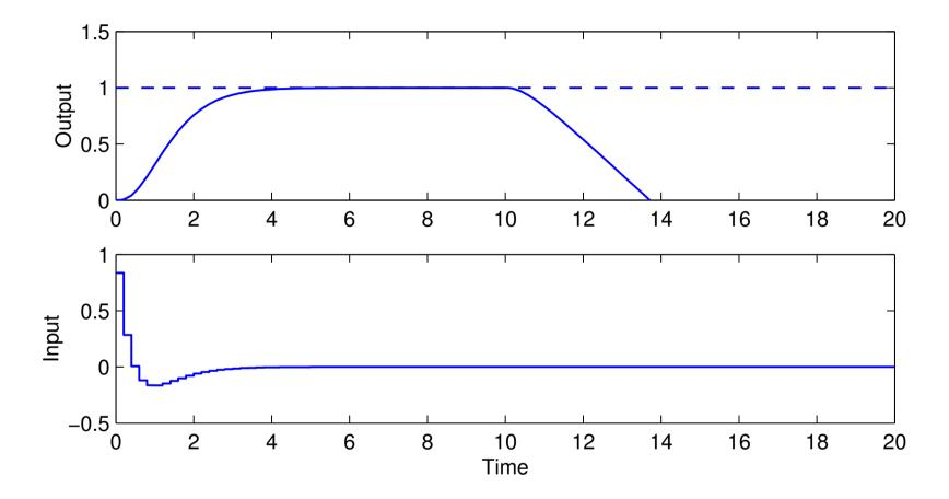
Does not work – the feedback is needed to handle the load disturbance
