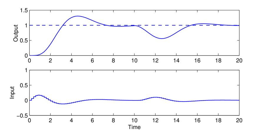
Does not work very well – the feedforward term is needed to get the desired reference step response Simulation without the feedback term  $(u(k) = u_{ff}(k))$ :
