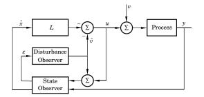
The disturbance estimator is integrating the prediction error of the observer.
