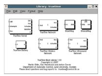
• A Kernel block, three Network blocks, and a Battery block
