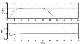
Does not work – the feedback is needed to handle the load disturbance
