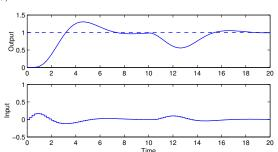
Does not work very well – the feedforward term is needed to get the desired reference step response Simulation without the feedback term  $ig(u(k)=u_{\it ff}(k)ig)$ :
