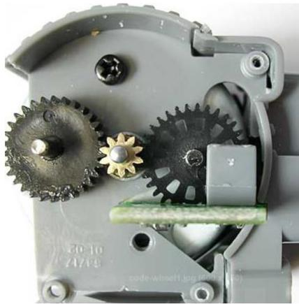
**Figure 3.2:** Encoder in motor
