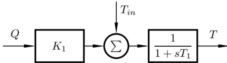
Response to step disturbance  $T_{in} = 1$  (suppose  $Q = 0$ ):
