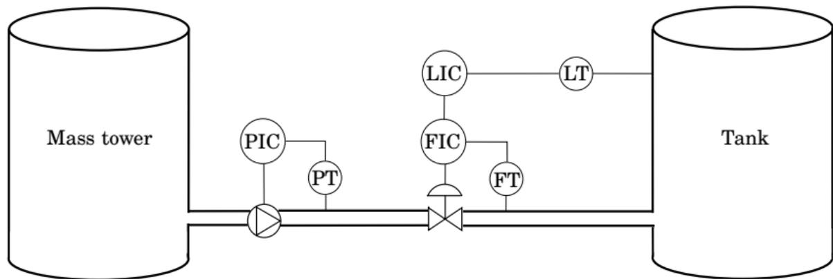
Pipe pressure to be kept constant, while desired flow decided by tank level controller
