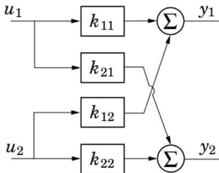
Closed loop gain from  $u_1$  to  $y_1$  when all outputs controlled to zero except  $y_1$ :
