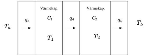
Two elements with thermal capacities  $C_1$  and  $C_2$  separated by insulating layers. Heat flows:  $q_3$ ,  $q_4$  and  $q_4$
