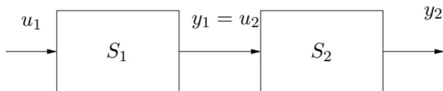
Block models (*à la* Simulink) often requires a predetermined causality which can be problematic. We want to be able to model in general without first determining what is input and what is output.
