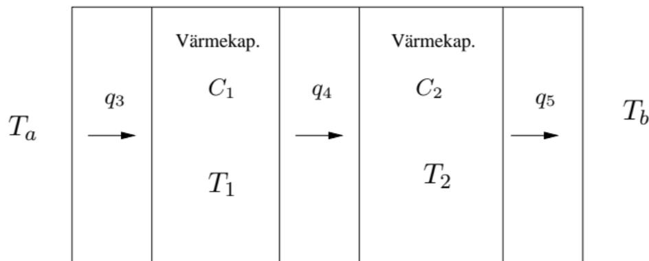
Two elements with thermal capacities  $C_1$  and  $C_2$  separated by insulating layers. Heat flows:  $q_3$ ,  $q_4$  and  $q_4$
