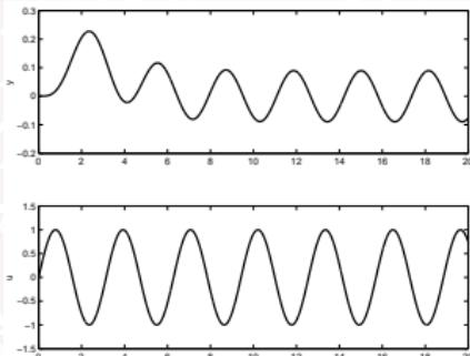
Sinusoidal input  $u(t) = u_0 \sin(\omega t)$  gives (if  $G(s)$  stable):
