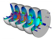
Control of electric field in accelerator cavity.
