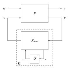
Find stabilizing *state observer/state feedback* controller. Augment the stabilized system with Q-parameter in special way (Boyd et al. 1991; Megretski 2011).
