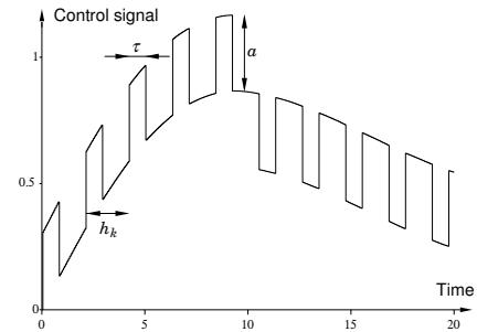
Add short pulses to the control signal in the direction of the rate-of-change.
