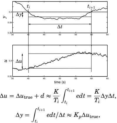
$$\Delta u = \Delta u_{\text{true}} + d \approx \frac{K}{T_i} \int_{t_i}^{t_{i+1}} edt = \frac{K}{T_i} \Delta y \Delta t,$$
