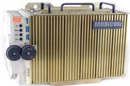
Figure 4: The Modicon 184, second programmable controller of Modicon.
