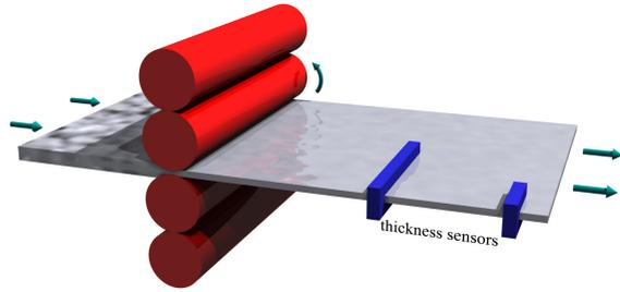
Thickness can only be measured at some distance from rolls, leading to
