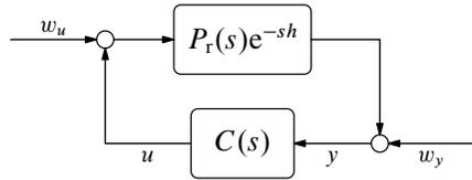
This feedback system called internally stable if transfer matrix  $\begin{bmatrix} w_y \\ w_u \end{bmatrix} \mapsto \begin{bmatrix} y \\ u \end{bmatrix}$ ,
