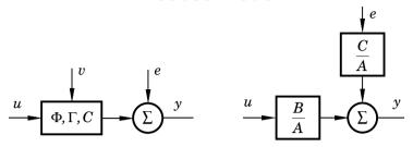
Two noise sources. Reduce to one (for  $R_{12} = 0$ )
