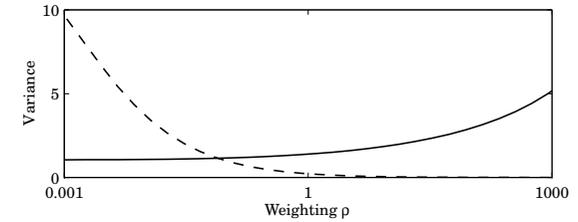
**Figure 12.8** Variances of input  $u$  (dashed line) and output  $y$  (solid line) for LQG controllers having different values of the control weighting  $\rho$  for the system in Example 12.10
