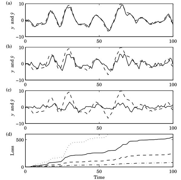
**Figure 12.3** The process output (dashed) and the predicted output (solid) for Example 12.3 when (a)  $m = 1$ , (b)  $m = 3$ , (c)  $m = 5$ , and (d) the accumulated prediction loss,  $\sum (y(k) - \hat{y}(k | k - m))^2$ , for  $m = 1$  (dashed-dotted),  $m = 2$  (dashed),  $m = 3$  (solid), and  $m = 5$  (dotted).
