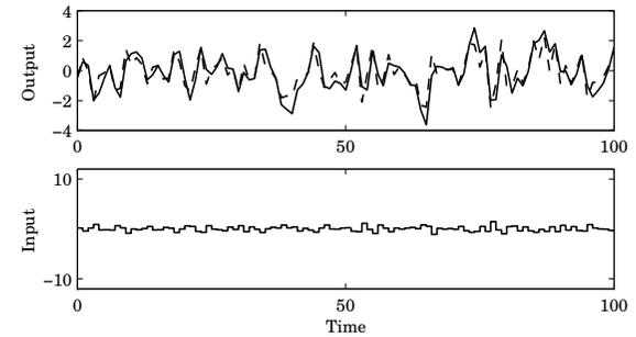
**Figure 12.9** Simulation of the for the system in Example 12.10 using the LQG-controller with  $\rho = 1$ . The output obtained with the minimum-variance controller ( $\rho = 0$ ) is shown in dashed. Also compare with Fig. 12.6.
