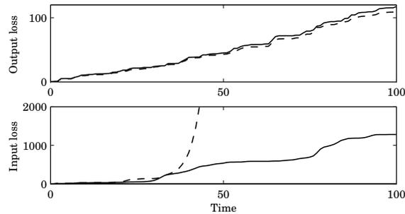
Figure 12.7 The accumulated output loss  $\sum y^2(k)$  and input loss  $\sum u^2(k)$  when the controllers (12.31) (solid) and (12.27) (dashed) are used.
