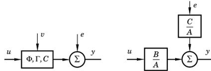
**Figure 12.1** Representation of a system with one input and stochastic disturbances using one or two noise sources.
