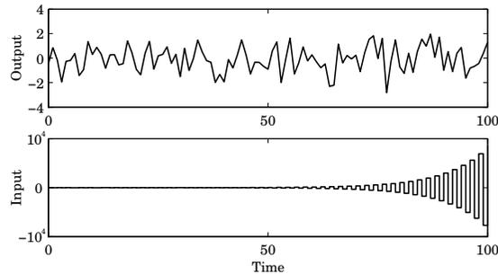
**Figure 12.5** Simulation of the system in Example 12.8 with the control law given by Theorem 12.2 that cancels an unstable process zero.
