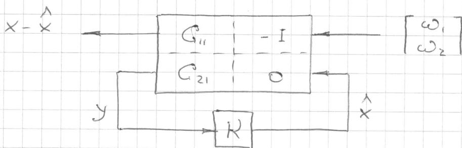
$$\text{with } G_{11} = \left[ \begin{array}{c|cc} A & Q_x^{1/2} & 0 \\ \hline 1 & 0 & 0 \end{array} \right], \quad G_{21} = \left[ \begin{array}{c|cc} A & Q_x^{1/2} & 0 \\ \hline C & 0 & Q_y^{1/2} \end{array} \right]$$
