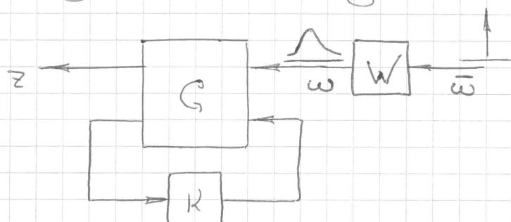
Minimizing the  $H_2$  norm from  $\bar{\omega}$  to  $z \Leftrightarrow$  minimizing the energy of the response of  $z$  to  $\Delta$  in  $\omega$ .
