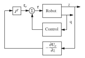
Unless the constrained system is strictly positive real (SPR), the gain margin has a **finite upper limit**, thus restricting the application of artificial potential feedback.
